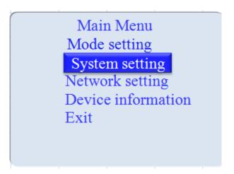
The system settings in the LCD menu can be used to set the displayed language, screen brightness, backlight time and reset. After pressing the system settings, the menu is displayed (as shown below).
