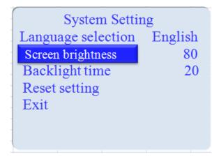
The LCD backlight time can be set in the brightness of 5-100 after pressing the backlight time:
