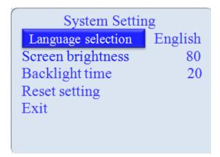
After pressing the screen brightness, you can set the LCD screen brightness in 10-100 brightness:
